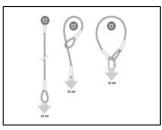
It offers several configurations for setting up an anchor: directly to an anchor point or around a suitable structure.
